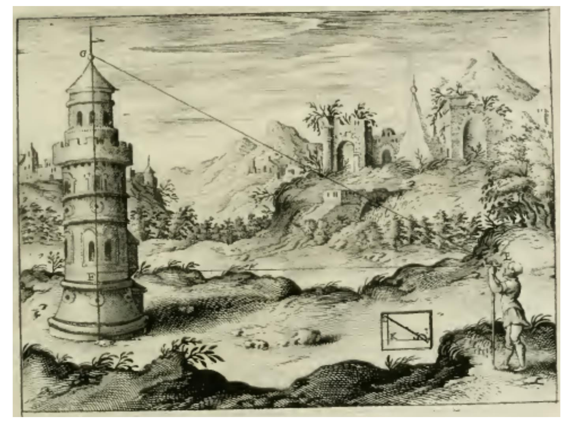
Using the graphometer to measure height
