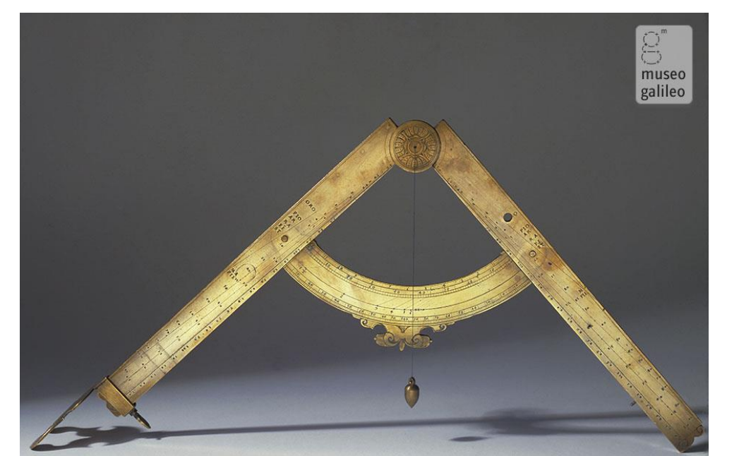
Proportional compass of Galileo (Galileo Museum in Florence): a true handheld calculator!
